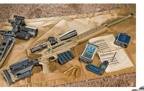
The .375CT SuperSport XLR features a patented continuous full length MIL-STD 1913 40MOA monolithic 12 o'clock scope rail design that increases structural rigidity and accommodates a variety of modern "clip-on" thermal imaging and night vision devices. The Quattro Alloy Series SuperSport forend features a heat venting design with repositionable 12" and 4" accessory rail locations on the ergonomically shaped forend at 3, 6 and 9 o'clock positions.
